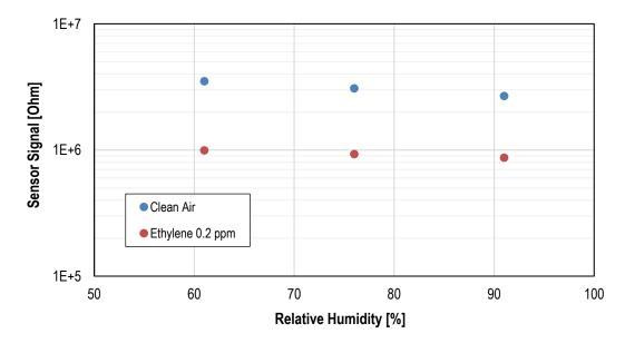
Figure 3. Humidity Influence at 4°C for Ethylene Stimulation
