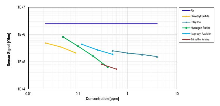
IDT provides firmware and algorithms, which allow the ZMOD4450 to learn the refrigeration environment. The gas sensor module will immediately respond to changes in the refrigeration air by detecting changes in the relative gas concentrations. When a user-defined threshold is exceeded, an I/O control signal (trigger) based on the algorithm output can be used to control an external device.
