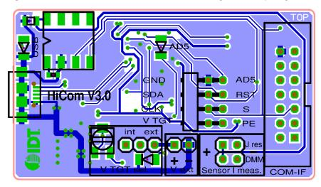
Figure 11. HiCom Communication Board Layout - Bottom Layer
