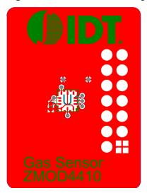
Figure 13. Sensor Board Layout – Bottom Layer
