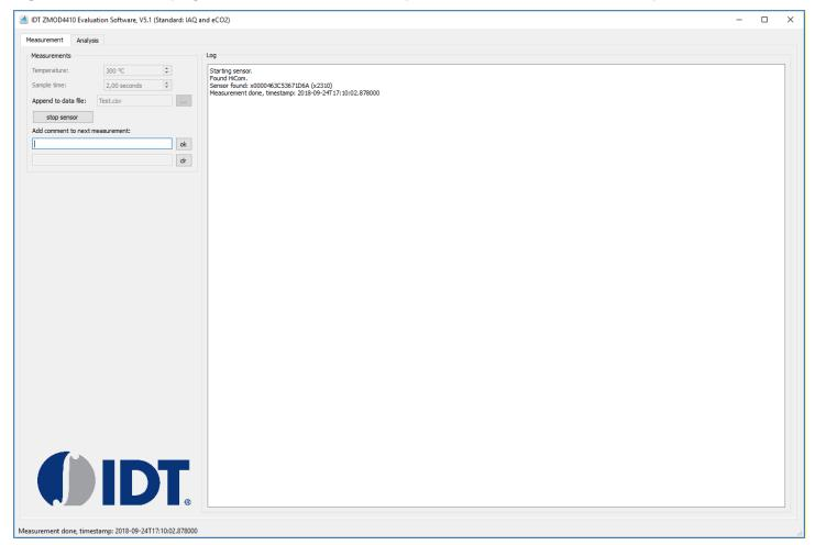
On the "Measurement" tab, the user can control the properties of the ZMOD4410's gas measurements. When the "start sensor" button is clicked, the measurement starts running continuously with the given sample time (2 seconds fixed for Standard Operation, 5 seconds (default) for Odor Operation, and 6 seconds fixed for Low Power Operation). IDT sets 300°C as the default temperature.
