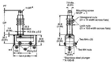
**Note:** Unless otherwise specified, a tolerance of  $\pm 0.8$  mm applies to all dimensions.
