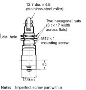
maximum length of 1.5 mm. Note: Do not use the M12 mounting screw and the case mounting hole at the same time, or the case may be damaged.
