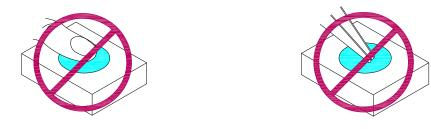
3. Do not stack together assembled PCBs containing exposed LEDs. Outside impact may scratch the silicone lens or damage the internal circuitry.
