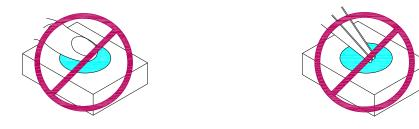
3. Do not stack together assembled PCBs containing exposed LEDs. Impact may scratch the silicone lens or damage the internal circuitry.
