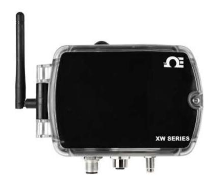
The XW Series Transmitters provide a wireless interface to a range of digital probes, digital I/O, and analog process signals. The radio is an IEEE 802.15.4 compliant transmitter operating at 2.4 GHz designed to transmit up to 1000 m\* (3280') and 100 m\* (328') to a ZW-REC coordinator.
