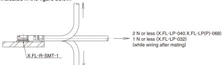
When the cable is routed in such a direction that lifts the cable, it is recommended that cushioning should be placed on the plug to prevent the connector from unmating (see the example below).
