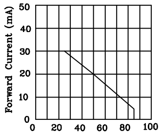
Ambient Temperature T_A ( ^\circ\text{C} ) FORWARD CURRENT DERATING CURVE
