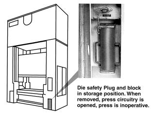
The receptacle is wired in-line with the machine control circuitry. The shorting plug is secured to safety equipment by a short length of chain. When the internally jumpered plug is engaged, it completes the circuit permitting the equipment to function.
