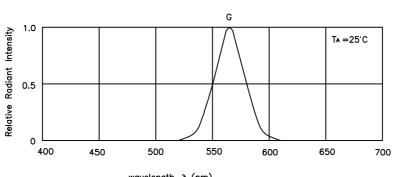
wavelength  $\lambda$  (nm) RELATIVE INTENSITY Vs. WAVELENGTH
