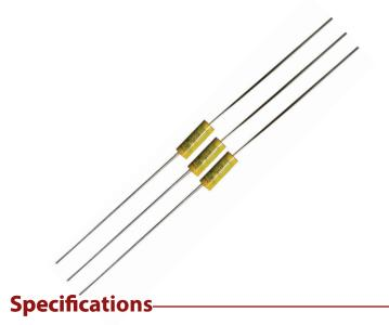
Type WMC axial-leaded polyester film/foil capacitors are ideal for automatic insertion in printed circuit boards. It is an ultraminiature version of Type WMF and the sections of these non-inductive capacitors are constructed with extended foil, polyster film, with tinned copper-clad steel leads.
