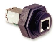
To bring Ethernet into a cabinet or control box, simply create the sealed connection on the outside of the enclosure, and run a commercial patch cord from the backside RJ-45 jack to your PLC, I/O, or Ethernet Control Board. No conduit entry is required.
