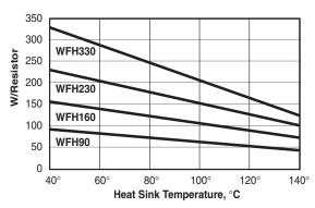
This graph shows the maximum wattage rating for each of the five possible ressistors of standard size corresponding to the heat sin temperature. It is assumed that all resistors are equally loaded. Please consult us about non-standard lengths and resistor modules.
