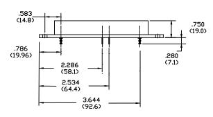
Do not use wire heavier than #22 WG. Excess stress on terminals could cause damage to internal components
