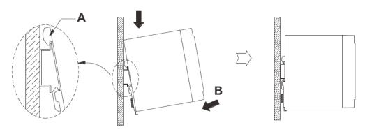
Firstly hang A part on the top of Rail as shown in below, then push the power supply into B direction to fix it.
