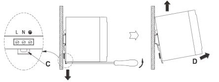
Remove the power supply to D direction, pulling C part by using tools, such as a screwdriver, to downward direction.
