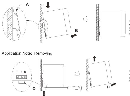
Firstly hang A part on the top of Rail as shown in below, then push the power supply into B direction to fix it.
