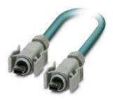
Assembled FireWire cable, shielded, color: RAL 5021 (water blue), PUR outer sheath, FireWire/IP67 on FireWire/IP67, length: 5 m
