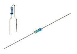
A metal glazed film is deposited on a high grade ceramic body. After a helical groove has been cut in the resistive layer, tinned electrolytic copper wires are welded to the end-caps. The resistors are coated with a light blue lacquer which provides electrical, mechanical, and climatic protection.
