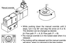
will return, when it is returned to the free position. Note) Be sure to release the locking before starting the normal operation
