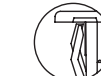
DETAIL VIEW VH1, VH3 & VH5 HOLE PLUGS (No wing serrations for ease of removal)
