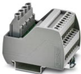
VARIOFACE module, with two equipotential busbars (P1, P2) for potential distribution, for mounting on NS 35 rails. Module width: 50.0 mm
