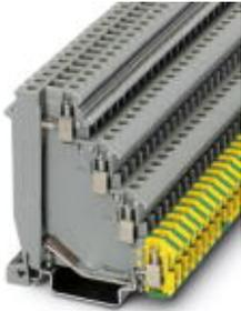
Sensor/actuator terminal block, Cross section: 0.2 mm<sup>2</sup> - 4 mm<sup>2</sup>, AWG: 24 - 12, Connection type: Screw connection, Width: 6.2 mm, Color: gray, Mounting type: NS 35/7,5, NS 35/15
