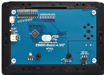
Figure 3-2 - VM800B module profile 4.3" display version
