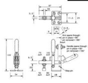
$\label{eq:continuous} \mbox{Adjustable spindle positioning along the arm with straight base. 100 daN holding force. Supplied with set screw, nuts, neoprene cover and flanged washers.}$
