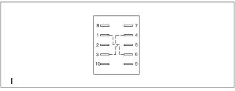
To have a polarity inversion (typical application: fan motor). Dotted line = internal wiring, continuous line = internal wiring
