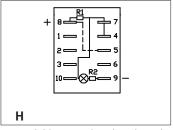
To obtain 2 symbol illumination levels (night illumination when OFF and higher illumination when ON). Dotted line = external wiring, continuous line = internal wiring
