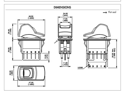
**Dimensions**: First dimensions are in mm while inches are shown as bracketed numbers.
