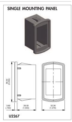
Recommended panel thickness: 1,10 mm - 1,80 mm - 2,60 mm - 3,40 mm - 4,20 mm - 5 mm - 5,80 mm
