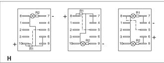
To obtain 2 symbol illumination levels (night illumination when OFF and higher illumination when ON).
