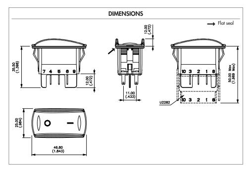
**Dimensions**: First dimensions are in mm while inches are shown as bracketed numbers.
