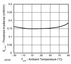
Fig. 10 - Sensitivity vs. Ambient Temperature
