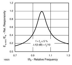
Fig. 5 - Frequency Dependence of Responsivity
