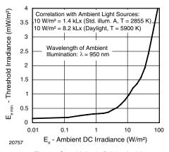
Fig. 6 - Sensitivity in Bright Ambient
