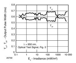
Fig. 4 - Output Pulse Diagram
