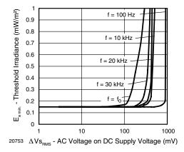
Fig. 7 - Sensitivity vs. Supply Voltage Disturbances
