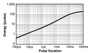
Limit of acceptance is a shift in resistance of less then 1% from the initial value. 100 joule Energy rating is for 10 mSec pulse width; for shorter pulses energy rating has to be derated according to above rating chart
