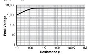
TRHE1 are tested in accordance with IEC61000-4-5, waveform 1.2/50ms, 10 pulses applied. Limit of acceptance is a shift in resistance of less then 1% from the initial value.
