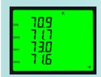
Extech's 12-Channel datalogging thermometer allows for a wide-range of applications with 6 Thermocouple types (J, K, E, T, R,S). It displays CH1 to CH8 or CH9 to CH12 on screen and data can be recorded from all 12 channels simultaneously onto an SD card in Excel<sup>®</sup> format for further analysis.
