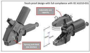
Maximum current rating20 AConnector to clip resistance10m ohmClip capacity:52 mm to 7 5mm with sliding jaw
