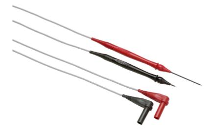
One pair (red, black) of test leads with sharp needle point tips adjustable to desired length from 0 to 76 mm, Extra hard probe tips to provide long service life, Flexible silicone insulated test leads, CAT III 300 V, 3 A rating, UL listed
