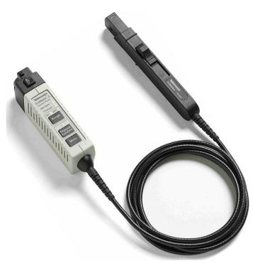
TCP0030A is a high-performance, easy-to-use AC/DC current probe designed for use and direct connection to oscilloscopes with the  $\mathsf{TekVPI}^\mathsf{TM}$ probe interface. This AC/DC current measurement probe provides greater than 120 MHz of bandwidth with selectable 5 A and 30 A measurement ranges. It also provides exceptional low-current measurement capability and accuracy to current levels as low as 1 mA, important for meeting today's challenging current measurement needs.
