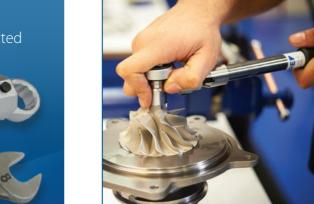
Improved accuracy, consistency and control. Accurate process control is ensured by reducing the risk of under and over tightening, due to unique Breaking Technology. This gives the operator more time to react once the target torque is reached
