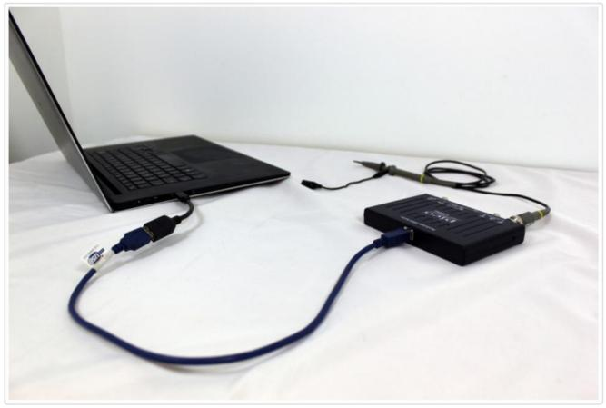
PicoScope 2208B connected to USB Type-C
