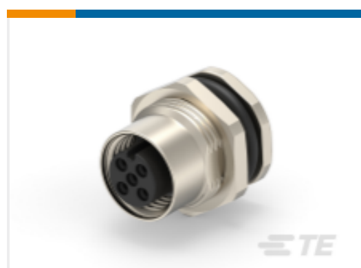
TE Part # T4131012031-001 M12,REAR MOUNT,FEMALE,A,3P, SOLDER WIRE
