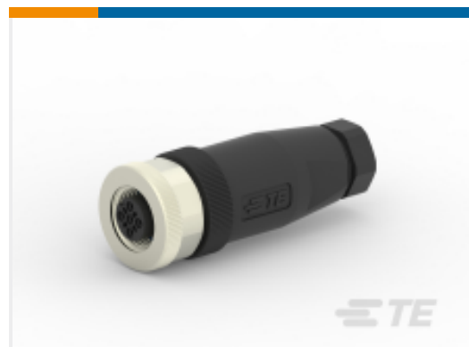
TE Part # T4110001031-000 M12,FEMALE,STRAIGHT,A CODE,3P, PG7,GOLD
