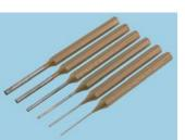
A set of 6 parallel pin punches made from Chrome Molybdenum steel for strength & durability. • Octagonal shank and a polished drift • Manufactured to DIN 6450 Contents: 2, 2.5, 3, 4, 5 and 6 mm
