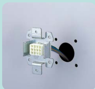
Drill a hole on the mounting surface of machinery.
