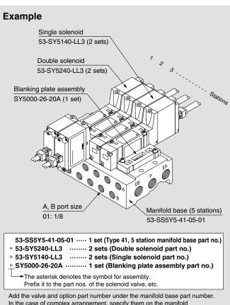
And the valve and option part number under the manifold base part nu In the case of complex arrangement, specify them on the manifold specification sheet.
