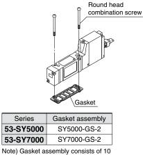
Iote) Gasket assembly consists of sets of mounting screws and gaskets.
