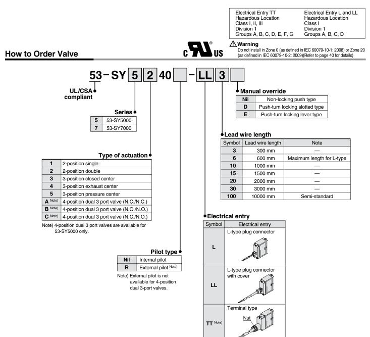
Note) The lead wire of TT-type is connected to the terminal block. Use only supplied cable and nut.
