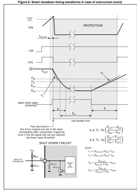
Note:  $R_{ON_{OD}}=V_{OD}/5$  mA see Table 11: "Sense comparator ( $V_{CC} = 15$  V, unless otherwise is specified)";  $R_{PD_{SD}}(typ) = 5$  V/I<sub>SDh</sub>.
