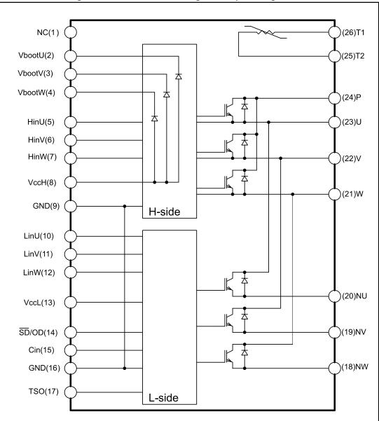
Figure 1: Internal schematic diagram and pin configuration
