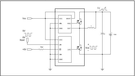
Figure 3: Switching time definition
