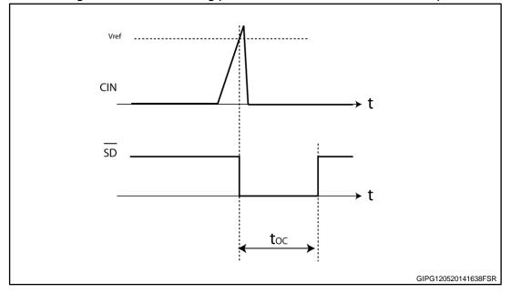
Figure 4: Overcurrent timing (without contribution of RC network on SD)
