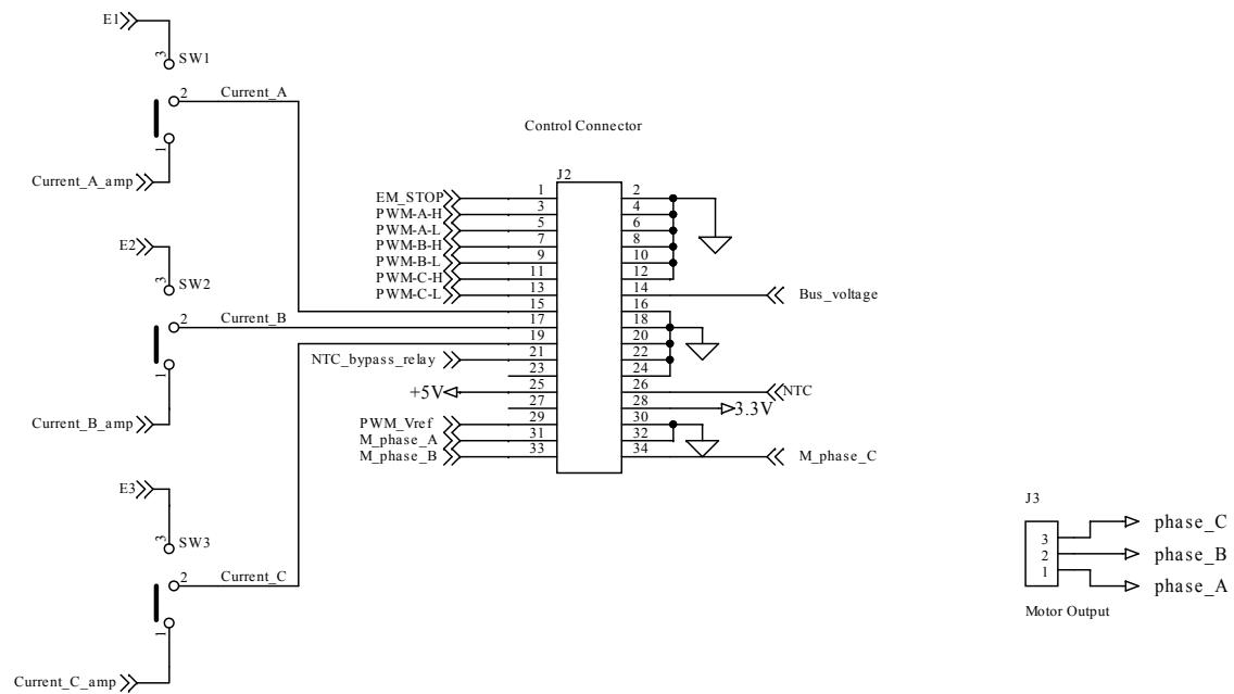
Figure 3. STEVAL-IPMNM3Q board schematic (3 of 5)
