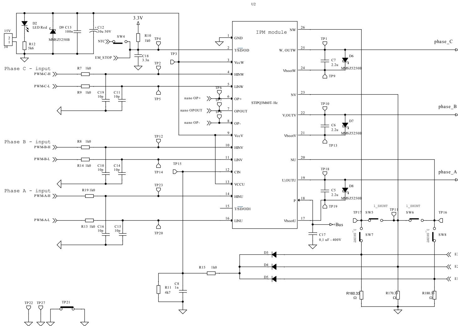
Figure 4. STEVAL-IPMNM3Q board schematic (4 of 5)
