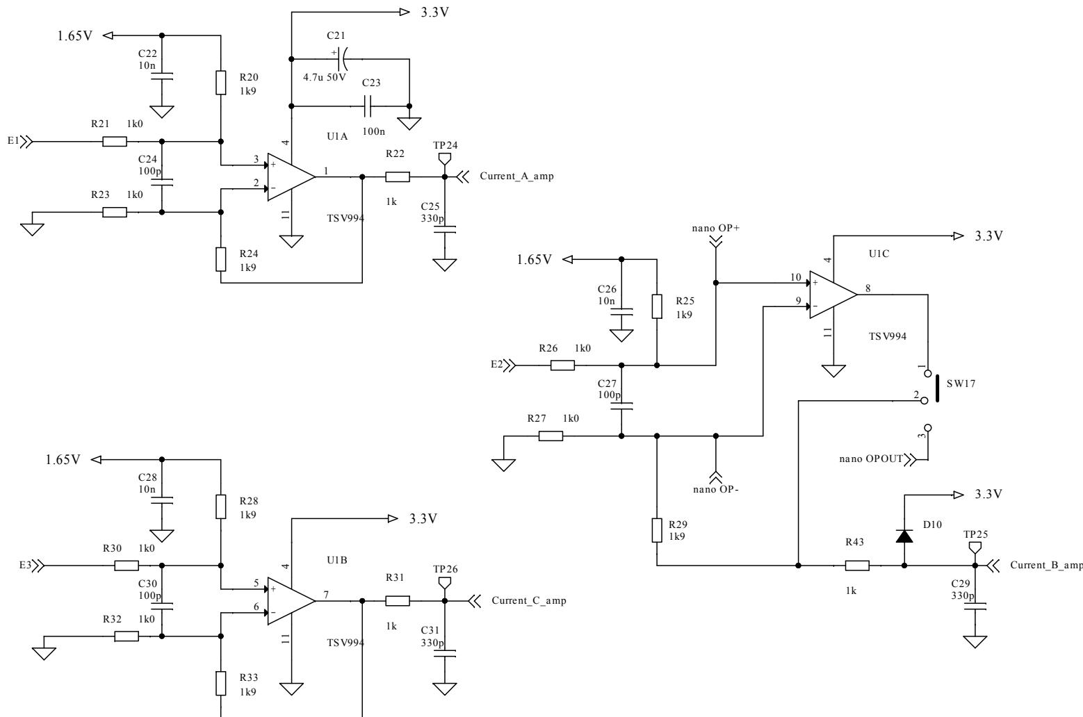
**Figure 5. STEVAL-IPMNM3Q board schematic (5 of 5)**
