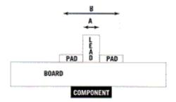
Select a tip cartridge with an inside diameter (A) larger than the lead diameter, and an outside diameter
