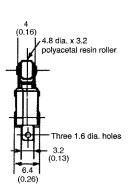
Note: Unless otherwise specified, a tolerance of  $\pm 0.4$  mm applies to all dimensions.
