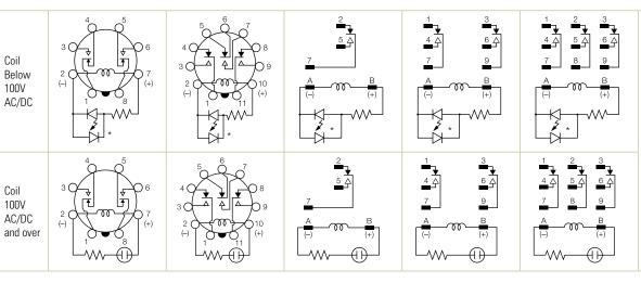
When the relay is energized, the indicator goes on.
