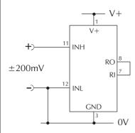
Measuring a single ended input voltage referenced to supply, i.e. the input voltage and the meter's power supply share the same 0V rail.
