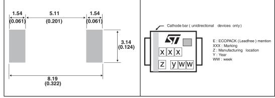
1. Marking layout can vary according to assembly location.
