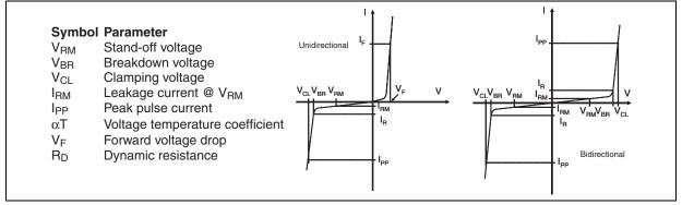
Figure 2. Pulse definition for electrical characteristics
