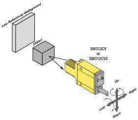
Distance from Sensor lens to object: 16 mm (0.65 in) for SM312CV 43 mm (1.7 in) for SM312CV2
