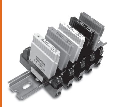
Pulse transformer technology for isolating I/O signals offers significant advantages over optical isolation and electromechanical relays. Most notably, pulse transformer I/O modules provide higher transient immunity and high input-to-output isolation.
