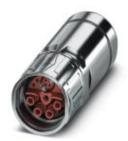
Cable connector, straight long, shielded: yes, SPEEDCON locking, M23, No. of pos.: 8+4+PE, type of contact: Socket, Crimp connection, cable diameter range: 9 mm ... 12 mm
