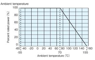
For resistors operated at an ambient temperature of  $70^{\circ}\!\mathrm{C}$  or higher, the power shall be derated in accordance with the above derating curve.
