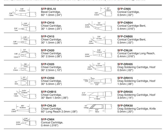
To order specialty versions of the Soldering Tip Cartridges replace the "F" in the part number with the appropriate letter designate for your application when ordering: T = Temperature Sensitive, C = Ceramic or Heavy Load
