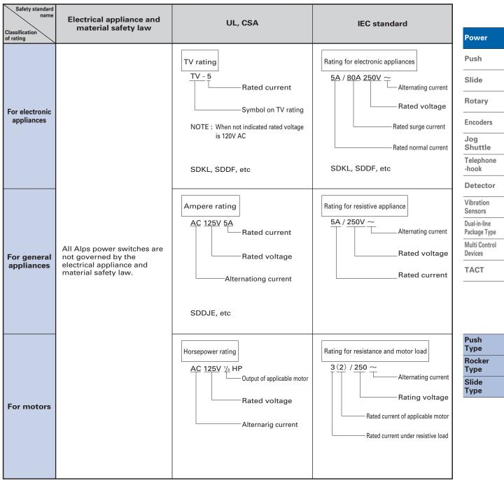
**Power switches for electronic appliances:** Mainly power switches for electronic appliances such as TV sets, radios and amplifiers. However, if the voltage and current levels are below the ratings, they may be used in other electric appliances.
